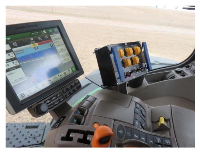
Customer has used a JD mobile phone bracket to support the Accuspray switch box.
